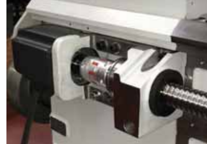
▲ Direct drive of the ballscrew
