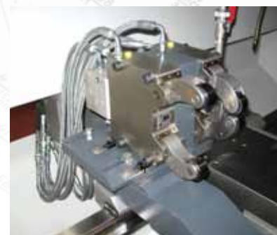
▲ Hydraulic self-centering follow dual rests – automatic tandem working
