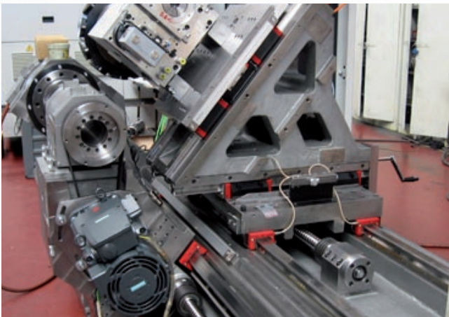
▲ Machine design is based on solid castings ensuring extreme rigidity during machining
