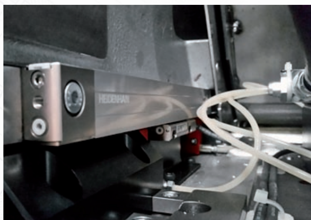
▲ Direct linear measuring increases accuracy of each working axis
