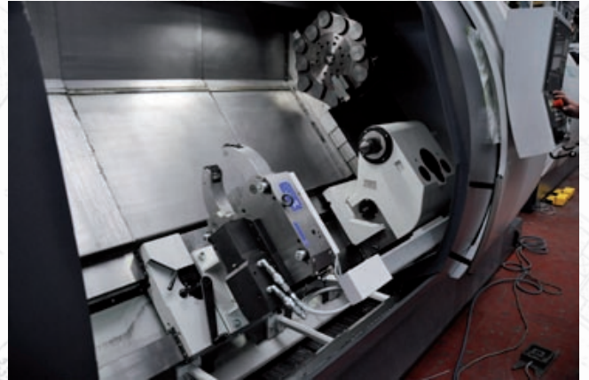
▲ Tailstock with hydraulic sleeve
