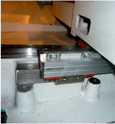
^ Linear measuring HEIDENHAIN
