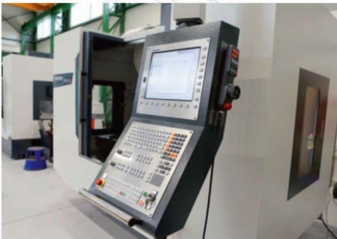
▲ Control system HEIDENHAIN TNC 640
