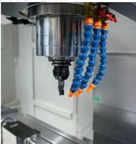
^ External cooling of the cutting tools
