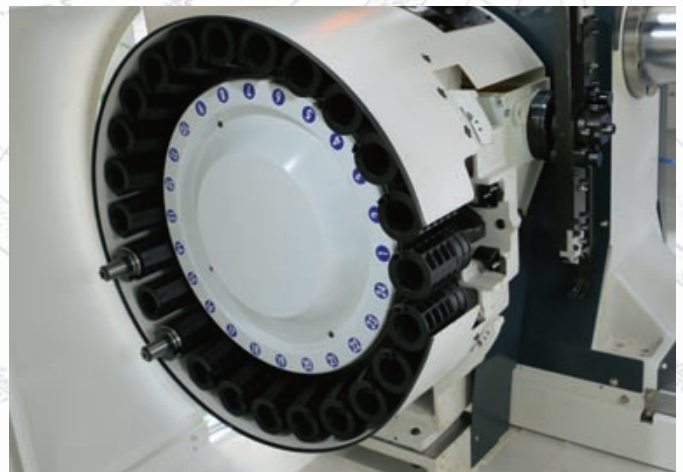
▲ Built-in tool magazine for 24 tools
